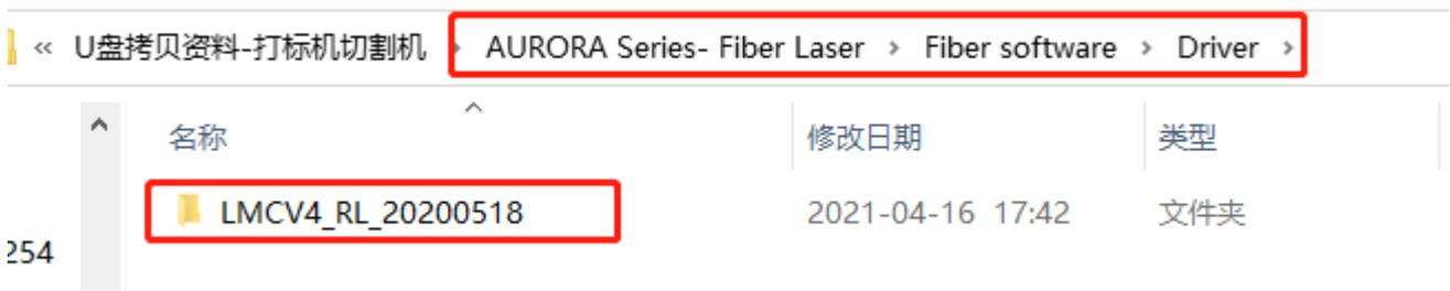
1. Go Manage>>Device manager>>Other devices>>USBLMCV2>>right click, Update driver>>Browse my computer for driver software>>Browse, and find the CV4 folder you saved from the U-disk that came with the fiber laser>>Select the CV4 driver>>Next>>Install, then the driver is installed successfully. See below pictures.
