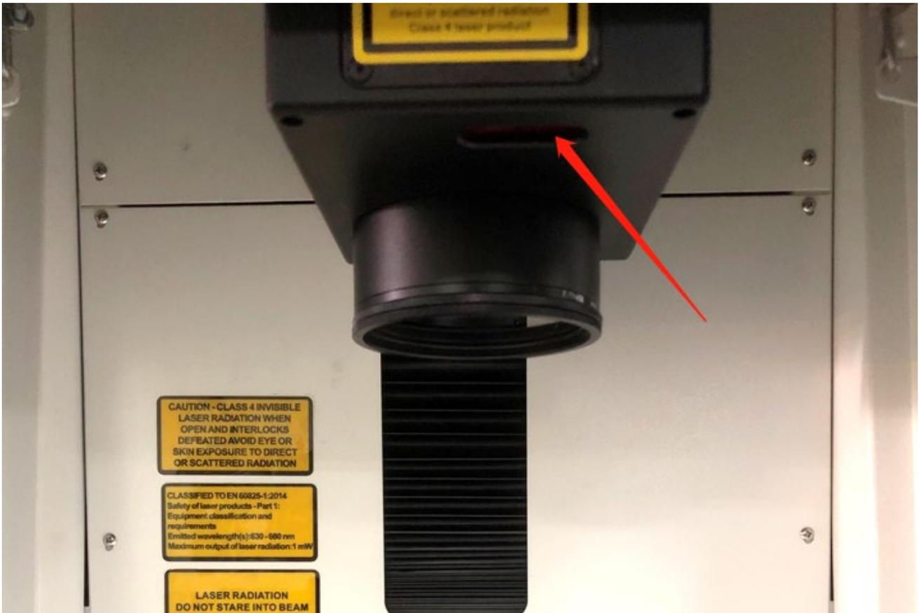
9. Press Key F1 or Red(F1) in software, then fiber will virtual marking out the size of your file. Adjust the position of your material according to the red area. See below pictures.
