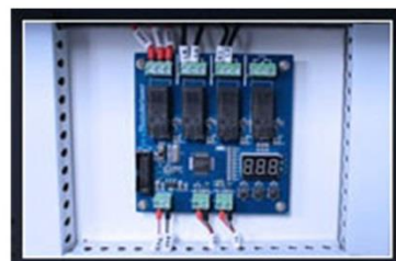
Smart Board Control the exhaust fan, air assist, and alarm lamp automatically, energy saving.
